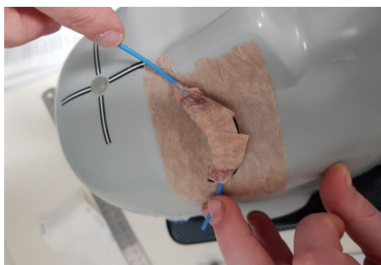
FIGURE 3-4 RED WAX ON PHANTOM, SHOWING GAPS AND POOR DELINEATION
