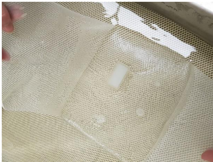
FIGURE 3-5 SOFTENING OF THERMOPLASTIC IN 70 DEGREE WATER BATH
