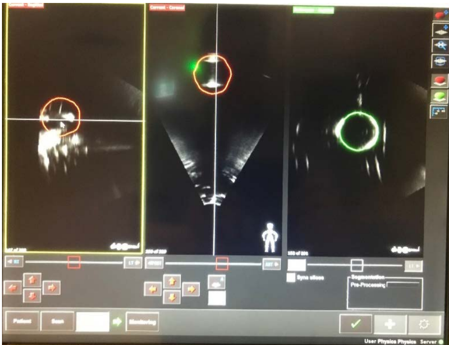
Figure 38: Clarity display showing tracking volume surrounding chamber thimble in sagittal (left) and coronal (centre) planes
