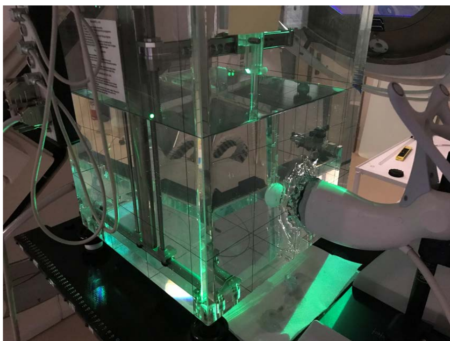
Figure 15: Experimental setup for verification of the 2D algorithm showing improved prostate analogue
