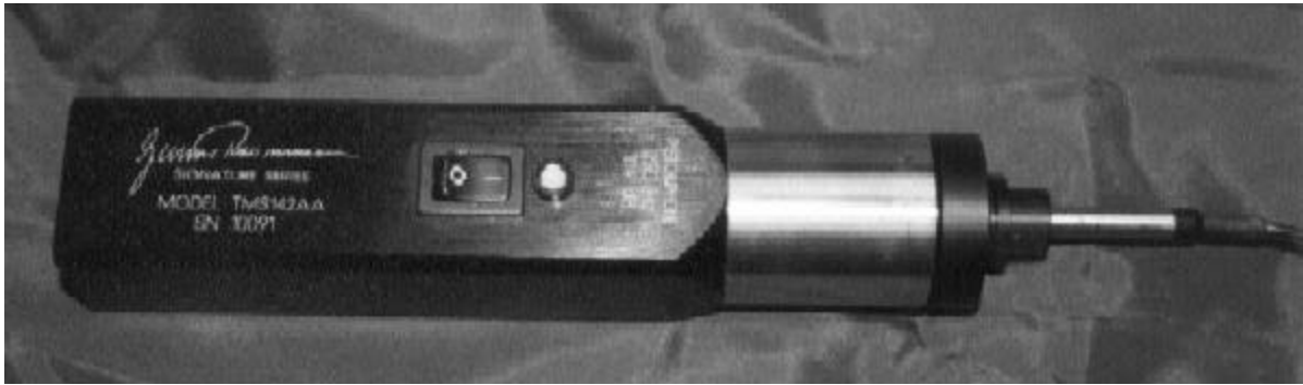
Figure 4.31 Pistonphone microphone amplitude calibrator. This instrument produces a constant sound pressure level of 114dB at 250 Hz.
