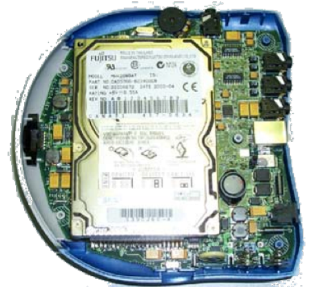
Creative Nomad Jukebox player- Internal view highlighting Fujitsu hard drive components
