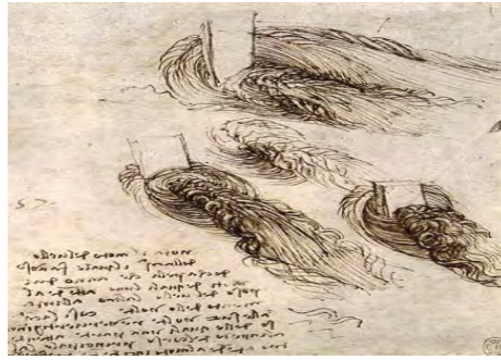
Figure 2.1: Sketch by Leonardo da Vinci in 1513 showing the wake behind a piling in a river (Garcia 2008).
