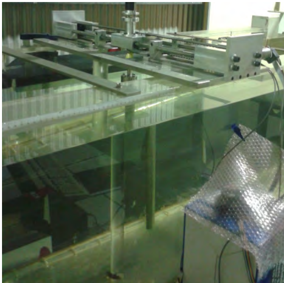
a) Water channel and VMSD model
