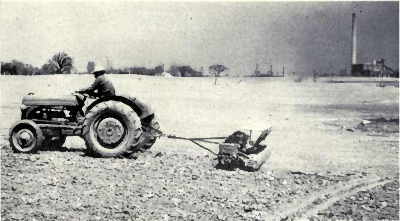
A multi-packer type of seeder has been used on mined lands because it makes a firm, fine seedbed and covers the seed. (Fig. 28)
