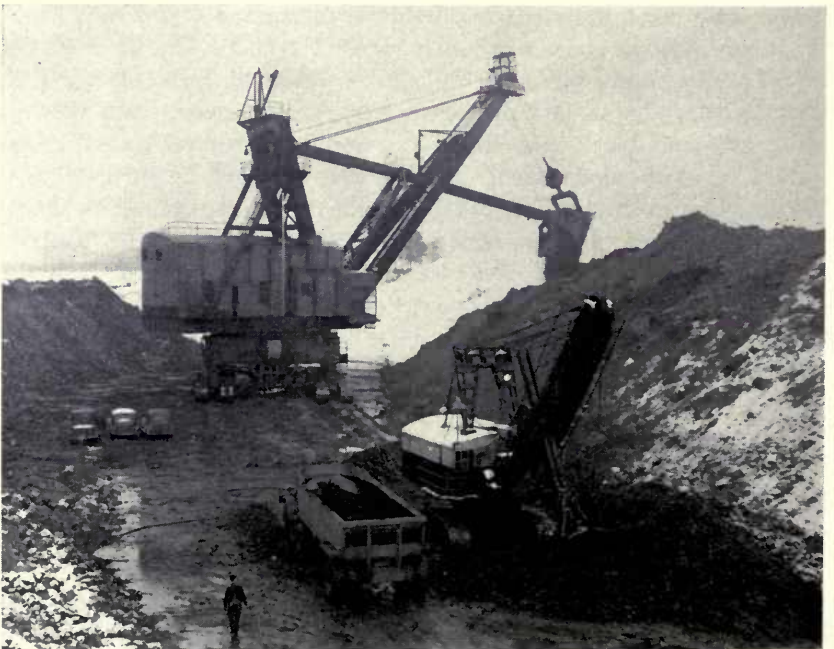
A modern 1600-ton stripping shovel in action. It has a 35-cubic-yard bucket and a 7-cubic-yard loading shovel. The haulage truck shown in foreground has a 40-ton capacity.
