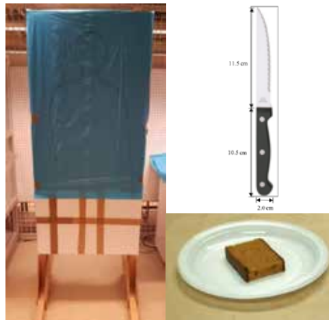
Figure 3.2: Stabbing construction (left), steak knife used in the experiments (right, up) and gingerbread used for the cutting scenario (right, down).
