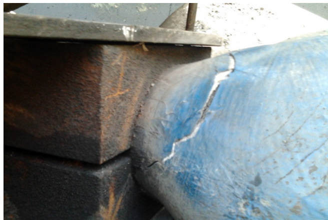
Figure 1: Failed fan blade at the neck portion [12]
