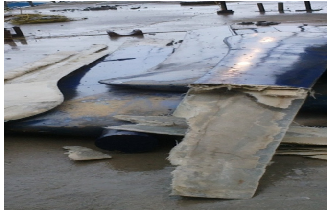
Figure 2. Failed fan blade at 1/3 of the blade length [12]
