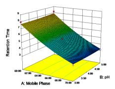
Fig. 2: Three-dimensional plot for retention time as a function of pH of buffer and amount of methanol. Constant factor (flow rate-1 ml min<sup>-1</sup>)
