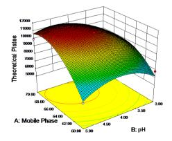
Fig. 4: Three-dimensional plot for theoretical plates as a function of pH of buffer and amount of methanol. Constant factor (flow rate-1 ml min<sup>-1</sup>)
