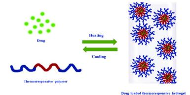
Fig. 2: The schematic representation of thermoresponsive hydrogel formation loaded with drug-using temperature as a stimulus [30]
