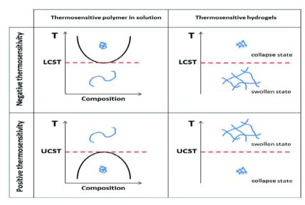
Fig. 3: Thermosensitive behaviors of polymers in solution and hydrogels [34]
