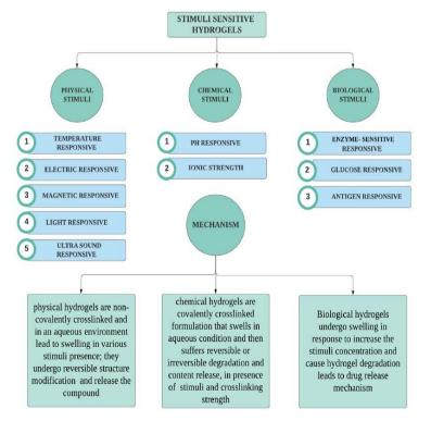
Fig. 1: Stimuli sensitive hydrogels and its mechanism [21]
