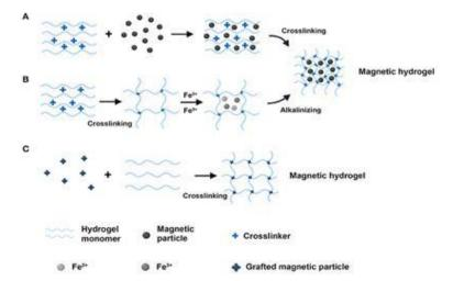
Fig. 4: The schematic diagram of the main three routes for the synthesis of the magnetic hydrogels. (A) The blending method. (B) The in situ precipitation method. (C) The grafting-onto method [42]
