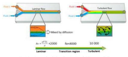
Fig. 6: Laminar and turbulent flow in microfluidic system [63]
