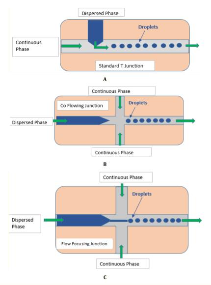
Fig. 4: Droplets microfluidic platforms (A) T-junction; (B) co-flowing junction and (C) flow-focusing junction [12]
