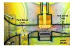
Fig. 5: bioMEMS microfluidic device actuated with 'microteeth' [57]
