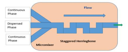
Fig. 3: Staggered herringbone mixer for the fabrication of microfluidic drug carriers [12]
