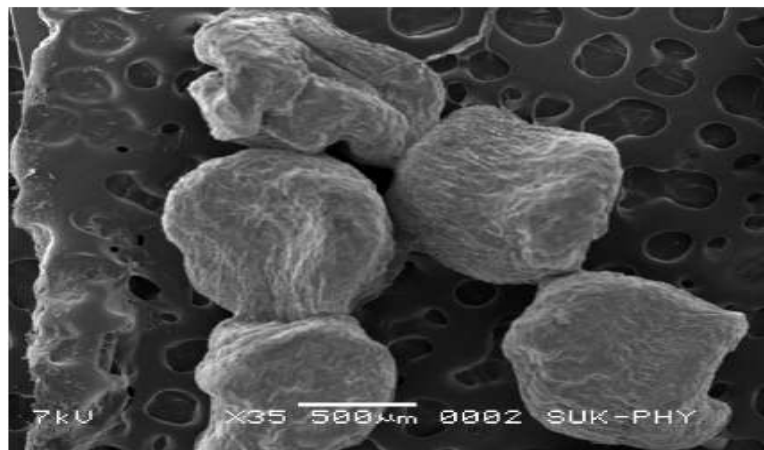
Fig. 11: Scanning electron microscopy (SEM) of ritonavir microbeads
