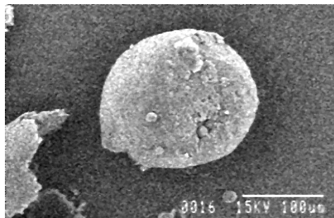
Fig. 6: SEM of cd microbeads under high resolution of X 300
