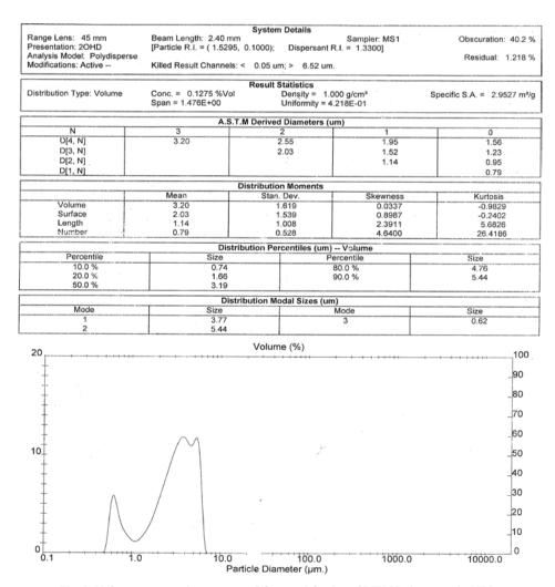
Fig. 3: Malvern mastersizer report of the particle size of REV SS niosomes in MDIs Note: D(4,N), D(3,N), D(2,N), D(1,N) are the equivalent derived diameter at 90, 80, 50 and 10% cumulative volume
