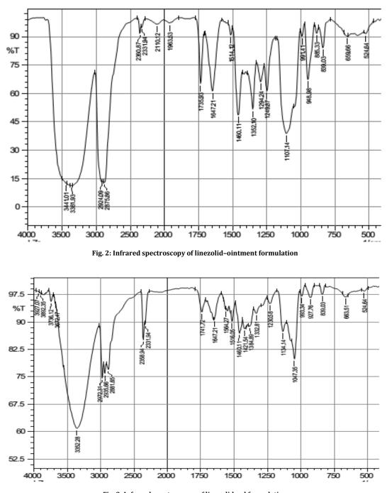
Fig. 3: Infrared spectroscopy of linezolid-gel formulation
