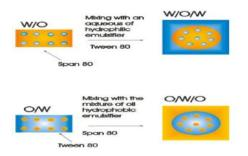
Schematic Diagram of W/O/W & O/W/OEmulsions
