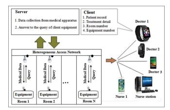
Fig. 1: The proposed system architecture of the health monitoring system using visible light communications transmission
