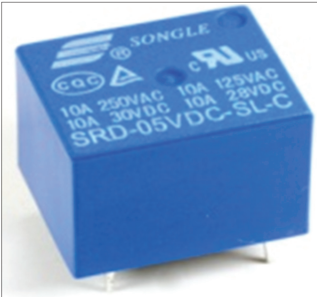
Fig. 8: Simple relay used in the proposed model
