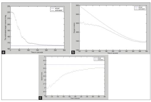
Fig. 1: (a) Error in course estimate, (b) error in range estimate, (c) error in speed estimate
