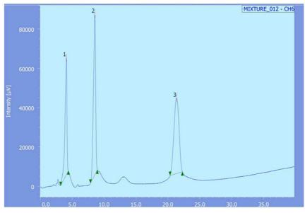
Fig. 6: HPLC chromatogram of a 20 μl injection of a standard mixture of 0.1 μg/ml TRT, 8 μg/ml HQ and 1 μg. ml<sup>-1</sup> HC using the optimized chromatographic conditions
