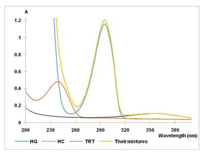
Fig. 4: Absorption curves of 40 µg. ml<sup>-1</sup> HQ in methanol, 10 µg. ml<sup>-1</sup> of HC in methanol, 0.5 µg. ml<sup>-1</sup> TRT in methanol and their mixture
