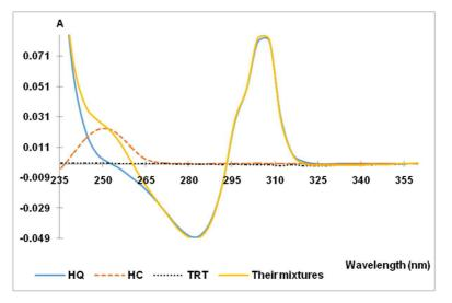
Fig. 5: D<sub>1</sub> spectra of 10 μg. ml<sup>-1</sup> HC in methanol, 40 μg. ml<sup>-1</sup> HQ in methanol, 0.5 μg. ml<sup>-1</sup> in methanol and their mixture
