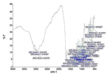
Fig. 3: FTIR spectra of usnic acid
