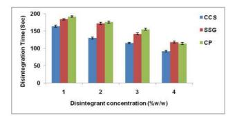
Fig. 1: Comparison of disintegration time of formulations prepared using different super-disintegrants (n=3, Mean=±SD)
