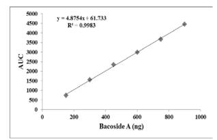
Fig. 3: Standard plot of bacoside A in TLC densitometric analysis.
