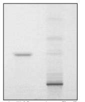
Fig. 2: Comparative TLC fingerprint profile of bacoside A and methanol extract of *B. monnieri* aerial parts under UV chamber at 254 nm
