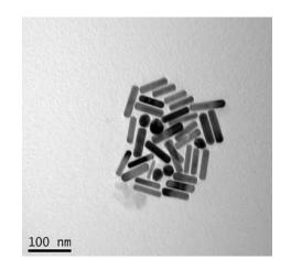
Fig. 1: TEM image of gold NRs with plasmon band energies at 800 nm
