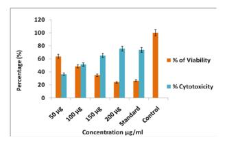
Fig. 6: Cell viability and cytotoxicity in A549 cells induced by exposure to different concentration of AgNPs determined by MTT assay
