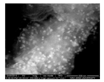
Fig. 5: FESEM showing spherical AgNPs synthesized from *S. samarangense* aqueous leaf extract
