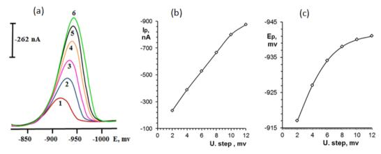
Fig. 5: The effect of voltage step (U. step) 2, 4, 6, 8, 10 and 12 mV and sweep rate (curves 1-6) on the polarograms (a),  $I_p$  (b) and  $E_p$  (c) of RSV (192.61 ng. mL $^{-1}$ ) using DPPM at HMDE (Purge gas  $N_2$ , Purge time 100 s, pH=1.5, t. meas 32 ms, U. amplitude -90 mV, t. pulse 35 ms, U. meas -300 mV, temperature 25°± 5°C and  $Na_2$ HPO<sub>4</sub> buffer)
