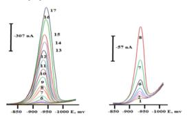
Fig. 7: The polarograms in the optimum conditions using DPPM on HMDE of RSV in  $Na_2HPO_4$  buffer (pH 1.5) at concentrations: 1- 0; 2- 0.9631; 3- 1.926; 4- 2.889; 5- 4.82; 6- 9.63; 7- 19.26; 8-38.52; 9- 48.15; 10- 72.23; 11- 96.31; 12- 120.38; 13- 144.46; 14- 168.54; 15- 192.61; 16- 240.75 and 17- 288.91 ng. mL-1
