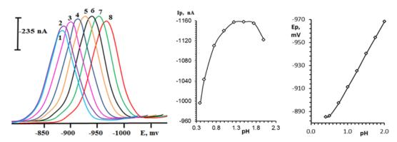
Fig. 1: The effect of pH solution at: 0.40; 0.50; 0.75; 1.00; 1.25; 1.50; 1.75 and 2.00 (curves 1-8) on the polarograms (a),  $I_p$  (b) and  $E_p$  (c) of RSV (192.61 ng. mL<sup>-1</sup>) using DPPM at HMDE (Purge gas  $N_2$ , Purge time 100 s, Scan rate 6.667 mV/s, U. amplitude -90 mV, U. step 10 mV, t. meas 32 ms, t. pulse 35 ms, t. step 1.5 s, U. meas -300 mV, temperature 25°± 5°C and  $N_{12}$ HPO<sub>4</sub> buffer)
