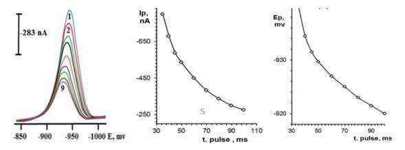
Fig. 3: The effect of time pulse (t. pulse) at: 35, 40, 45, 50, 60, 70, 80, 90 and 100 ms (curves 1-9) on the polarograms (a),  $I_P$  (b) and  $E_P$  (c) of RSV (192.61 ng. mL $^{-1}$ ) using DPPM at HMDE (Purge gas  $N_2$ , Purge time 100 s, Scan rate 6.667 mV/s, U. step 10 mV, pH=1.5, t. meas 32 ms, U. amplitude -90 mV, t. step 1.5 s, U. meas -300 mV, temperature 25°± 5°C and  $N_{12}$ HPO<sub>4</sub> buffer)
