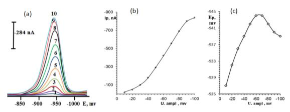
Fig. 2: The effect of negative pulse amplitude (U. ampl) at: -10; -20; -30; -40; -50; -60; -70; -80; -90 and -100 mV (curves 1-10) on the polarograms (a),  $I_p$  (b) and  $E_p$  (c) of RSV (192.61 ng. mL $^{-1}$ ) using DPPM at HMDE (Purge gas  $N_2$ , Purge time 100 s, Scan rate 6.667 mV/s, U. step 10 mV, pH=1.5, t. meas 32 ms, t. pulse 35 ms, t. step 1.5 s, U. meas -300 mV, temperature 25°± 5°C and  $Na_2$ HPO<sub>4</sub> buffer)
