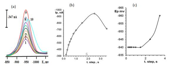
Fig. 4: The effect of time interval for voltage step (t. step) at: 0.2, 0.3, 0.4, 0.5, 0.6, 0.8, 1.0, 1.5, 2.5 and 3.5 s (curves 1-10) on the polarograms (a),  $I_p$  (b) and  $E_p$  (c) of RSV (192.61 ng. mL<sup>-1</sup>) using DPPM at HMDE (Purge gas  $N_2$ , Purge time 100 s, pH=1.5, t. meas 32 ms, U. amplitude -90 mV, t. pulse 35 ms, U. meas -300 mV, temperature  $25^{\circ}\pm5^{\circ}$ C and  $N_{10}\pm10^{\circ}$ C and  $N_{10}\pm10^{\circ$
