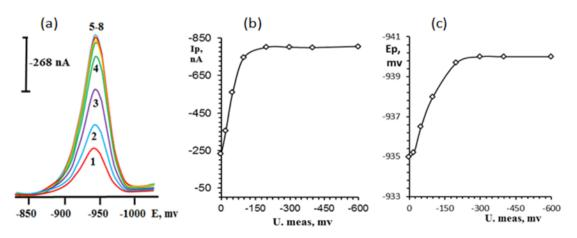
Fig. 6: The effect of U. meas 0, -20, -50, -100, -200, -300, -400 and -600 mV (curves 1-8) on the polarograms (a),  $I_p$  (b) and  $E_p$  (c) of RSV (192.61 ng. mL $^{-1}$ ) using DPPM at HMDE (Purge gas  $N_2$ , Purge time 100 s, Scan rate 6.667 mV/s, pH=1.5, t. meas 32 ms, U. amplitude -90 mV, t. pulse 35 ms, U. step 10 mV, t. step 1.5 s, temperature 25°± 5°C and  $Na_2HPO_4$  buffer)
