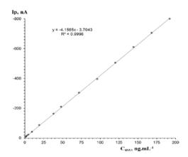
Fig. 8: Calibration curves for the determination of RSV using DPPM on HMDE under the optimum conditions.
