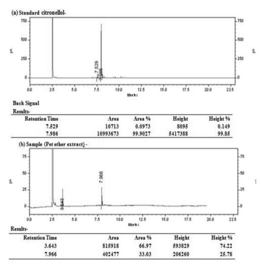
Fig. 3: Gas chromatogram of (a) standard citronellol and (b) pet ether extract
