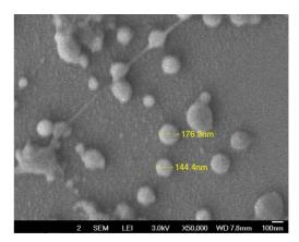
Fig. 2: SEM images of synthesized NZVI-CNS
