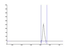
Fig. 2a: Chromatogram of Betulinic Acid with corresponding Rf value at 540 nm. Stationary Phase: HPTLC Plates coated with silica gel 60 F<sub>254</sub> Mobile Phase: Toluene:Ethyl Acetate: Methanol (16:2:2 v/v) Detection: Anisaldehyde Sulphuric Acid
