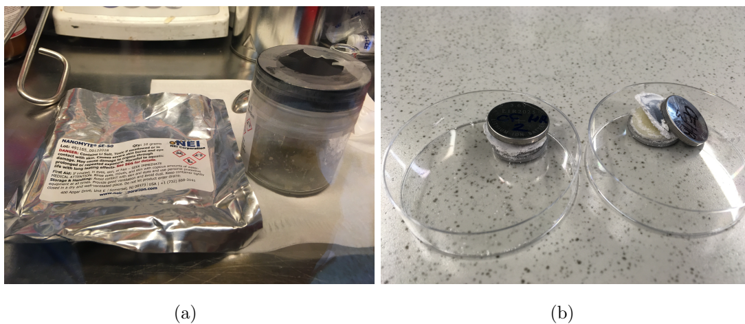
Figure 84 – a) commercial electrolyte nanomyte SE50, b) Li—nanomyte SE50—Li cells were bursting after several days.
