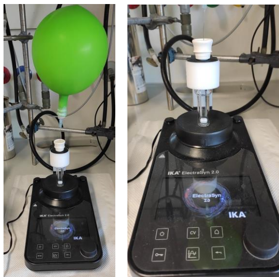
Figure 57. Electrochemical setup employed in the frame of the present thesis: IKA ElectraSyn 2.0 potentiostat with IKA vials (5 mL + 10 mL, in this picture: 5 mL vial) equipped with working and counter electrode, a septum on the outlet and an argon-filled balloon on top.
