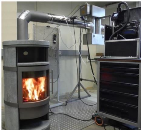
Figure 1. Pilot electrostatic precipitator downstream the stove.
