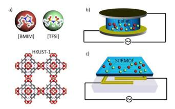
**Fig.1 a** Structure of [BMIM][TFSI] ionic liquid and HKUST-1 MOF. **b** and **c** Sketch of the setup for the conductivity measurement of IL@HKUST-1 MOF material in the form of a pellet sandwiched between two planar electrodes (**b**) and in the form of a thin film grown on a substrate with deposited electrodes, like interdigitated gold electrodes on glass sheets (**c**)
