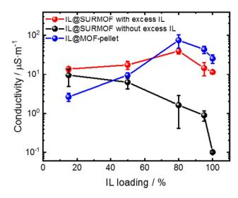
Fig. 6 Conductivity of [BMIM][TFSI] in HKUST-1 SURMOF film without excess IL and with excess IL on the surface and IL@MOF-pellet with different IL fillings
