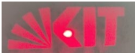
Figure 3: Photo of the transversely shaped laser on the screen of the test setup shown in Fig. 2. The zeroth order diffraction is visible in the center.
