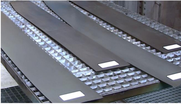
Figure 3. ODS steel plates after rolling. From the second block, two 2 mm and two 3 mm thick plates were produced by hot and cold-rolling.
