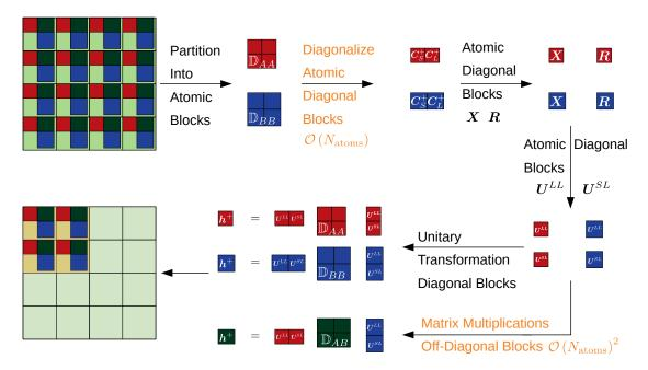
Figure 2.2: Workflow of the DLU-X2C transformation. A molecule consisting of different atoms is assumed. N<sub>atoms</sub> denotes the number of atoms. The scaling of the CPU time is reported for most time-consuming steps. The most demanding steps are denoted by orange color.
