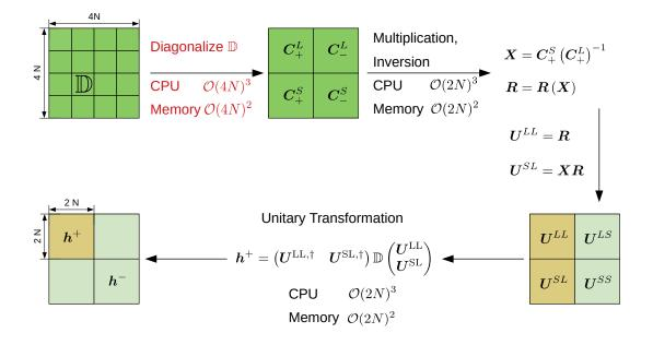
Figure 2.1: Workflow of the X2C transformation. N denotes the number of basis functions. The scaling of the CPU time and the memory demands are reported for the individual steps. The most demanding step is denoted by red color.
