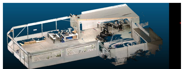
(b) Point cloud data of the Living-Lab
