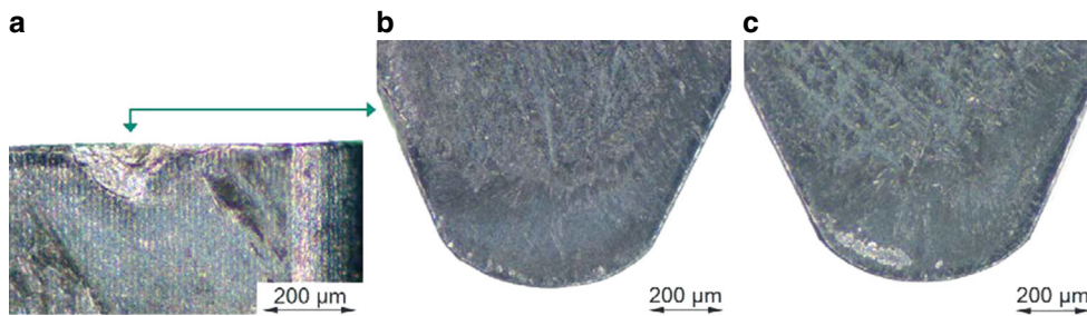
Fig. 10 Different wear characteristics for machining strength class R_m = 1,400 MPa in dry condition applying different process strategies with a cutting speed of v_c = 140 m/min. a LF—Strategy C 172 gaps manufactured b Rake face—Strategy C 172 gaps manufactured c Rake face—Strategy A 138 gaps manufactured
