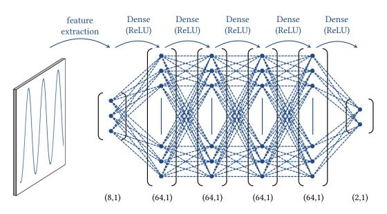
Figure 7.19.: Layout of the actor network used to process the observations defined by the eight-dimensional feature vector derived from the CSR power signal.
