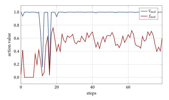
Figure 7.27.: Actions chosen by the PPO agent for the sequence displayed in Fig. 7.25. While the modulation frequency is dynamically adjusted according to the changing micro-bunching dynamics, the modulation amplitude is set close to the maximum value throughout the episode.
