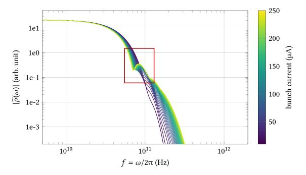
Figure 5.7.: Magnitude of the Fourier transformed bunch profile  $|\tilde{\rho}(\omega)|$  for a range of bunch currents below the instability threshold of  $I_{\text{th}} = 260 \,\mu\text{A}$ . The red rectangle marks the additional frequency component (at roughly 85 GHz) that is excited due to the perturbation by the CSR wake potential.
