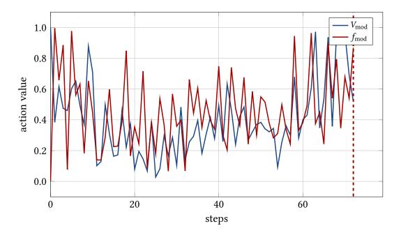
Figure 7.22.: Actions chosen by the DDPG agent during the sequence displayed in Fig. 7.20. Besides a slight trend to smaller action values halfway through the episode, the modulation amplitude and frequency mainly display rapid, irregular oscillations.
