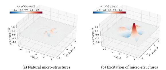
Figure 7.6.: (a) The naturally occurring set of micro-structures consists of about five structures with relatively small amplitudes. (b) An RF amplitude modulation at the third harmonic of the nominal synchrotron frequency,  $f_{\rm mod} = 3.06 f_{\rm s,0}$ , and with  $V_{\rm mod} = 0.05 V_0$ , leads to a new set micro-structures in the longitudinal phase space, which consists of only three structures, but of much larger amplitude.
