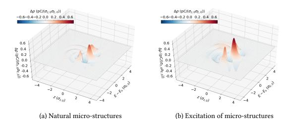
Figure 7.3.: (a) The naturally occurring micro-bunching dynamics lead to the formation of distinct micro-structures in the longitudinal phase space. (b) An RF amplitude modulation at the micro-structure frequency,  $f_{\text{mod}} = f_{\text{ms}}$ , and with  $V_{\text{mod}} = 0.05 V_0$ , leads to an amplification of the already naturally occurring structures by nearly 50 percent.
