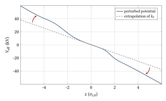
Figure 5.13.: The dynamic perturbation of the slope of the effective potential at the synchronous position  $k_0$  is found to be critical for the micro-structure formation process. By modulating the RF amplitude, the CSR-induced perturbation can be partially counteracted.
