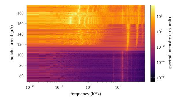
Figure A.1.: Shown is the same CSR Power Spectrogram as in Fig. 3.6 but with a logarithmic frequency axis, highlighting the low frequency contributions emerging around  $I = 120 \,\mu$ A.
