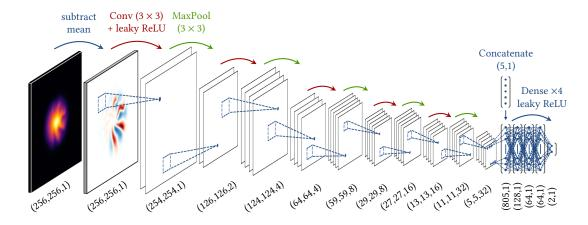
Figure 7.13.: Layout of the actor network used to process the states defined by Eq. (6.27). The charge density matrix is processed by alternating convolution and max pooling layers and subsequently concatenated with the additional feature vector, which serves as the input for the final fully connected layers.
