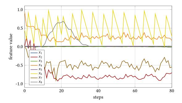
Figure 7.29.: Features as observed by the PPO agent. The termination condition is calculated using the proxies defined in Eq. (6.31) and Eq. (6.33). After an initial adjustment period, the phase difference between the applied RF amplitude modulation and the observed CSR power signal is kept almost constant by the agent, that is,  $x_7 \approx -0.5$ .
