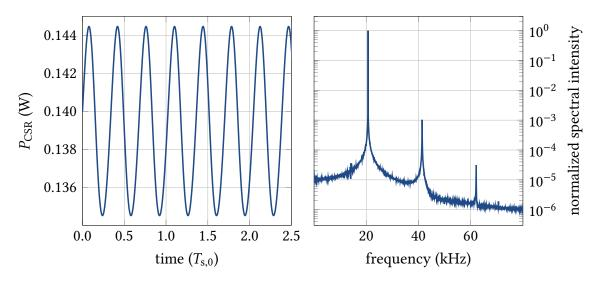
Figure 3.5.: CSR power time signal  $P_{\text{CSR}}(t)$  for the exemplary bunch current  $I = 115 \,\mu\text{A}$  (left) and the magnitude of its Fourier transform  $|\tilde{P}_{\text{CSR}}|$  (right).
