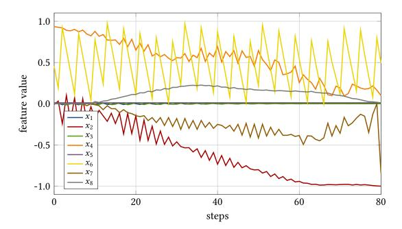
Figure 7.12.: Observed features corresponding to the sequence displayed in Fig. 7.8, calculated according to the definitions in Eqs. (6.13)–(6.21) and Eq. (6.35). The reduced standard deviation of the CSR power signal, encoded in feature  $x_2$ (red line), is the main reason for the high rewards achieved towards the end of the sequence.
