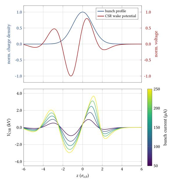
Figure 5.2.: CSR wake potential for a Gaussian bunch profile (red and blue, top) and for the bunch currents  $I = (50, 100, 150, 200, 250) \mu A$  below the instability threshold of  $I_{\text{th}} = 260 \,\mu A$  (bottom). Shown are the respective temporal averages for simulations (including damping and diffusion) of the parameter settings defined for  $\mathcal{D}_2$  in appendix A.1 (with  $g = 32 \,\text{mm}$ ).
