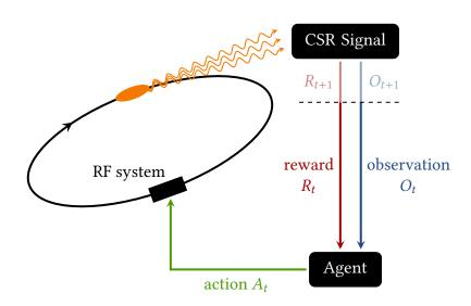
Figure 6.1.: General feedback scheme for the implementation of RL-based micro-bunching control at KARA. The agent receives an observation  $O_t$  and reward  $R_t$  calculated based on the measured CSR power signal  $P_{\text{CSR}}(t_i)$  and choses an action  $A_t$  that defines the RF amplitude modulation for the subsequent time step.
