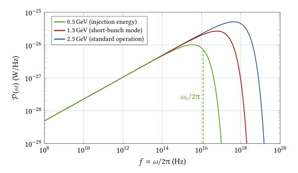
Figure 2.2.: Radiated power spectrum  $\mathcal{P}(\omega)$  of a single electron passing through a bending magnet (R = 5.559 m) for the typical beam energies at KARA. The green dashed line marks the critical frequency  $\omega_c$  at injection energy, it divides the power spectrum into two sections of equal integrated radiation power.
