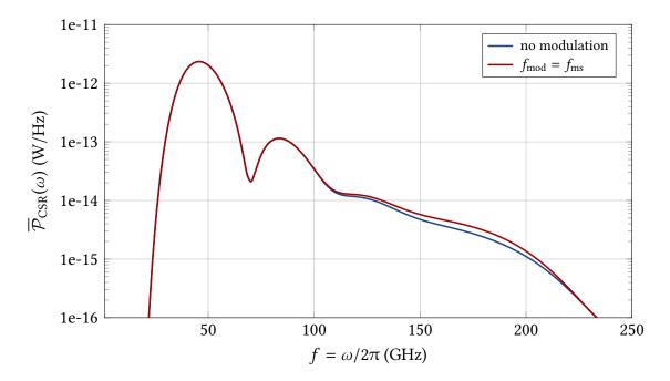
Figure 7.4.: The applied RF amplitude modulation amplifies the average CSR power spectrum in the frequency range corresponding to the spatial extent of the occurring micro-structures. Here, the emitted power is increased by up to 30 percent in the frequency range around 150 GHz.
