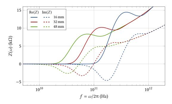
Figure 3.3.: CSR parallel plates impedance for different vacuum gaps. It describes the selfinteraction of an electron bunch with its own emitted CSR under the shielding effect of the surrounding vacuum chamber walls. A reduced vacuum gap leads to a stronger shielding, which shifts the cut-off frequency due to the beam pipe to higher frequencies. The beam pipe installed at KARA has a total height of g = 32 mm (red curves).
