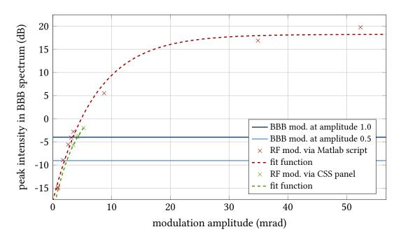
Figure 8.2.: Estimate of the BBB cavity voltage. By comparing the effect of RF phase modulations via the main RF system and the BBB system, the maximum BBB cavity voltage can roughly be estimated using Eq. (8.2). The measurements are interpolated by fitting a limited growth function,  $f(x) \doteq a - (a - b) e^{-cx}$ . Data: Courtesy of Edmund Blomley.
