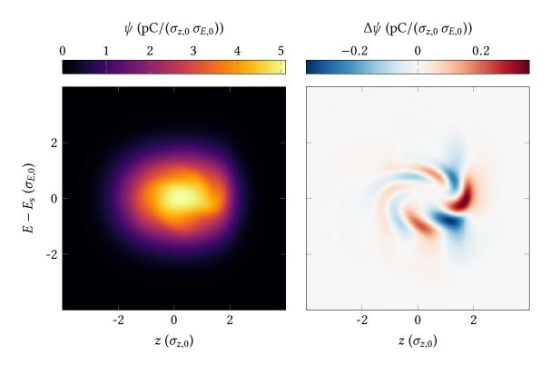
Figure 3.8.: Snapshot of the charge distribution in phase space in the regular bursting regime (left). The deformations of the distribution are emphasized by the subtraction of the temporal average, revealing a characteristic pattern of micro-structures (right).
