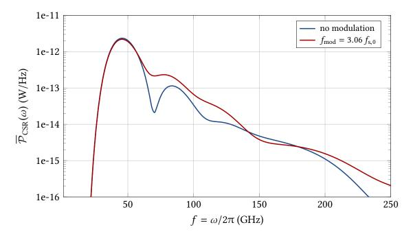
Figure 7.7.: The altered micro-bunching dynamics due to the applied RF amplitude modulation at  $f_{mod} = 3.06 f_{s,0}$  lead to substantial changes in the radiated CSR power spectrum. While the intensity is decreased in the frequency range corresponding to the spatial extent of the original micro-structure, the new set of large micro-structures shown in Fig. 7.6 increases the emission between 60 GHz and 140 GHz by a large margin.
