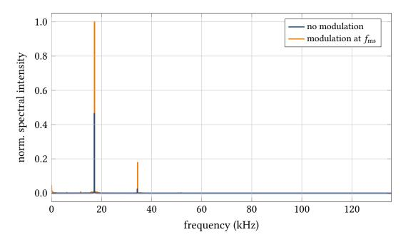
Figure 8.4.: Simulated fluctuation spectrum corresponding to the measurements in Fig. 8.3. The amplified peak intensity at  $f_{\rm ms}$  corresponds to an increased amplitude of the occurring micro-structures as illustrated in section 7.2.
