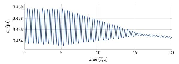
Figure A.6.: Evolution of the bunch length for the sequence displayed in Fig. 7.8. Both, the oscillation and the average value of the bunch length are decreased by the applied modulation of the RF amplitude.
