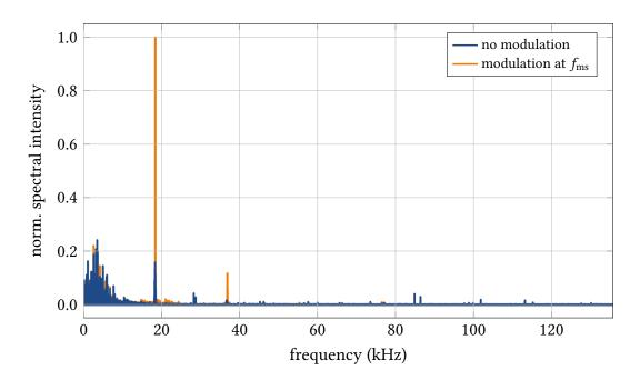
Figure 8.3.: Frequency distribution of the fluctuations in the measured CSR power signal. Besides low-frequency noise up to 10 kHz, the natural spectrum mainly features a distinct peak at the micro-structure frequency  $f_{\rm ms} = 18.45$  kHz. The applied RF amplitude modulation amplifies the spectral intensity of that frequency by more than a factor of five. The data may partially show oscillations of the arrival time at the THz detector. Data: Courtesy of Miriam Brosi.
