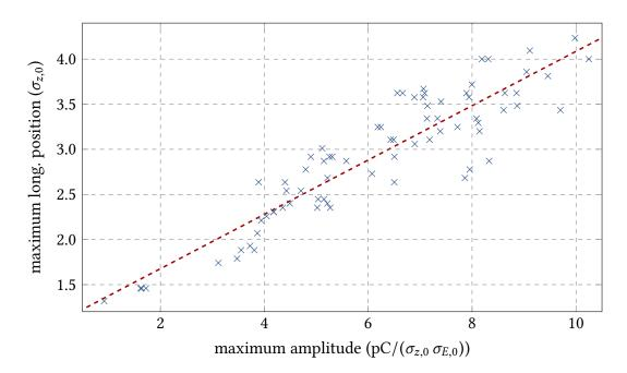
Figure 5.12.: Correlation between the maximum amplitude and maximum longitudinal position of the occurring micro-structures. Shown is simulation data for bunch currents between 260  $\mu$ A and 1000  $\mu$ A. The dashed red line illustrates the clear linear correlation with a correlation coefficient of 0.91.
