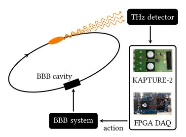
Figure 8.1.: Planned hardware implementation of the proposed RL feedback scheme. The CSR power signal is measured by a THz detector, sampled by the KAPTURE-2 board and read out by the FPGA DAQ board, on which the RL algorithm is implemented. The chosen action is passed to the BBB control system, which generates the corresponding modulation of the RF amplitude. Images: Courtesy of Weijia Wang.
