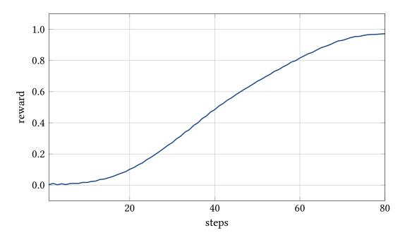
Figure 7.11.: Rewards corresponding to the sequence displayed in Fig. 7.8, calculated according to the definition in Eq. (6.30). To reduce oscillations in the reward signal, the CSR signal of four prior steps is used to calculate the mean and standard deviation.
