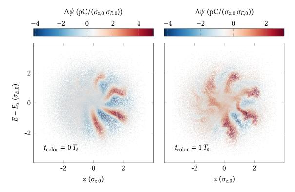
Figure A.5.: Analogously to Fig. 5.10, the particle distribution at time step  $t = 0 T_s$  is depicted with the color assignment  $\Delta \psi(q, p, t_{color} = 0 T_s)$  (left) and  $\Delta \psi(q, p, t_{color} = 1 T_s)$  (right) for the bunch current  $I = 500 \,\mu$ A. In contrast to the lower bunch current, the distributions show a partial overlap, indicating that particles stay within their respective structure over at least one synchrotron period.
