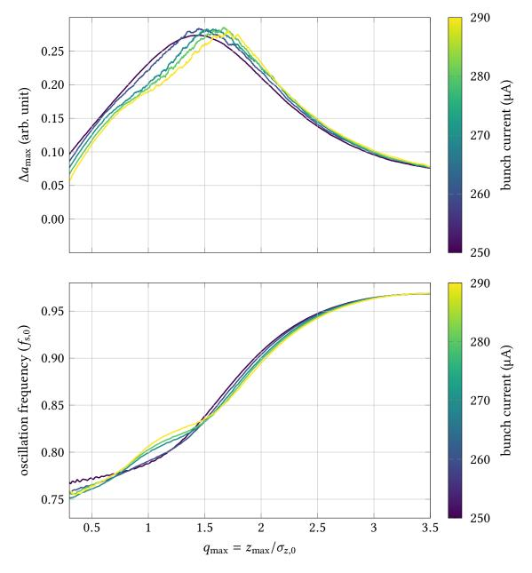
Figure 5.8.: Shown are the amplitude difference (top) and oscillation frequency (bottom) of particles trajectories for the bunch currents  $I = (250, 260, 270, 280, 290) \mu A$ . As the data scatters a lot, only a moving average over  $q_{\text{max}}$  is displayed to enable a comparison between different currents.
