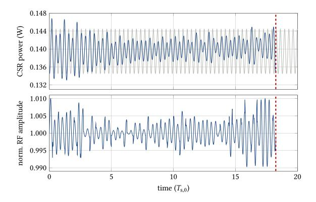
Figure 7.20.: Mitigation of the micro-bunching dynamics and the corresponding fluctuations in the CSR power signal (top) by the DDPG agent. The applied modulation of the RF amplitude (bottom) differs again from the manual control in Fig. 7.9b and also from that of the PPO agent in Fig. 7.14. The dashed red lines indicate the termination of the episode due to insufficient performance by the agent.
