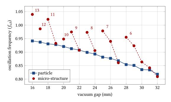
Figure 5.11.: Modifying the CSR shielding by varying the vacuum gap leads to altered micro-bunching dynamics in the longitudinal phase space. While the single particle frequency at the micro-structure position (blue squares) increases smoothly with reduced vacuum gap, the oscillation frequency of the micro-structures themselves (red circles) grows much faster and shows an abrupt change when an additional structure is observed.
