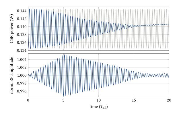
Figure 7.8.: Result of a carefully selected sequence of RF amplitude modulations, found in a trial-and-error process. The initial oscillation of the CSR power signal (top) is continuously damped by the applied RF modulation (bottom). At the end of the considered time frame, the oscillation of the CSR power signal is reduced to a minimum and clearly damped compared to the natural behavior of the instability indicated in gray.
