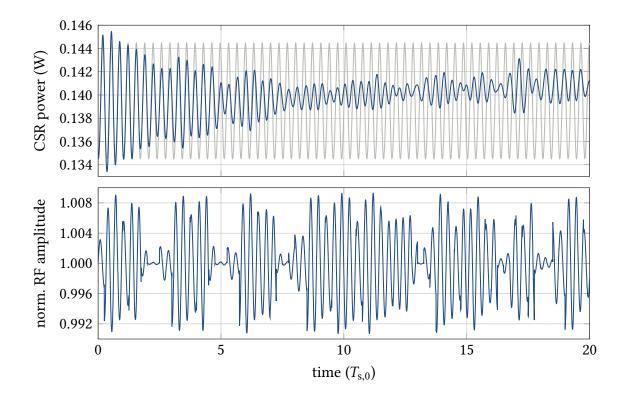
Figure 7.14.: Mitigation of the micro-bunching dynamics and the corresponding oscillations in the CSR power signal (top) by an RL agent trained with the PPO algorithm. The chosen actions and the resulting modulation of the RF amplitude (bottom) differ quite significantly from the manual control shown in Fig. 7.8. Yet, the agent clearly achieves a mitigation compared to the natural behavior of the instability (gray line) with an overall performance that is comparable.
