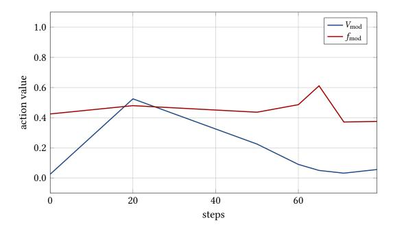
Figure 7.10.: Action values chosen during the sequence displayed in Fig. 7.8. The modulation amplitude  $V_{\text{mod}}$  is initially increased until the actions show the desired effect and the perturbation by the CSR wake potential is reduced. After the first 20 steps, it can therefore be lowered again. The modulation frequency is kept close to the natural micro-structure frequency at  $f_{\text{ms}} = 2.99 f_{\text{s},0}$ .
