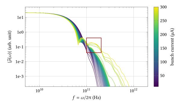
Figure A.4.: Magnitude of the averaged Fourier transformed bunch profile  $|\tilde{\rho}(\omega)|$  for a range of bunch currents. The peak at roughly 85 GHz corresponds to the quadrupole-like modulation already forming below the instability threshold of  $I_{\rm th} = 260 \,\mu$ A. The red rectangle marks the additional main frequency component that corresponds to the micro-structures forming in the longitudinal charge distribution.
