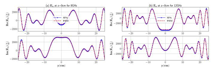
**Figure 7.** The real and imaginary part of the total electric field inside three-layer media with dimensions  $30 \text{ cm} \times 8 \text{ cm}$  and  $\epsilon_{r,1} = 1.16$  for the dielectric layer at 8 GHz and 12 GHz. Layer 2 is PEC.
