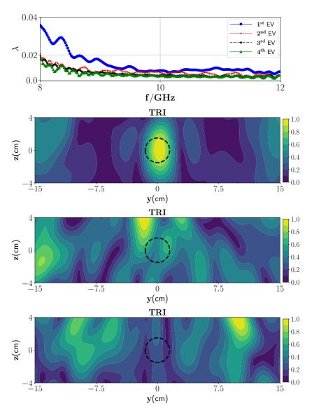
**Figure 5.** (**Top**) Magnitude of the first four eigenvalues versus the frequencies and (**second row**) reconstruction of one wet spot moisture case with TRI-DORT where the true location is marked by black dashed lines, (**third row**) reconstruction using third eigenvalue and its associated eigenvector, (**fourth row**) reconstruction using fourth eigenvalue and its associated eigenvector.
