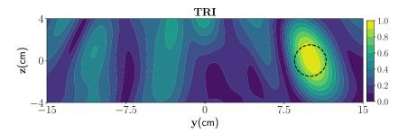
Figure 10. Reconstruction of one wet spot using TRI-DORT for moderate random rough surface.
