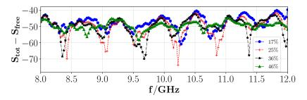
**Figure 12.** Experimental scattering response (in dB) in X-band of antenna 4 (middle antenna) for different moisture contents in the spherical wet spot of radius 1.5 cm.
