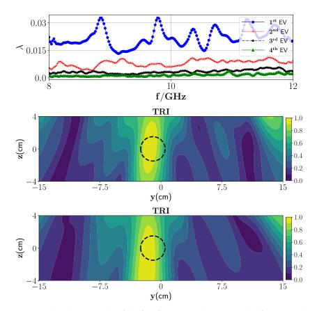
**Figure 13.** (**Top**) Magnitude of the first four eigenvalues versus the frequencies,(**middle**) TRI-DORT reconstruction image of one PTFE Teflon, and (**bottom**) SF-TRI-DORT at 8.07 GHz.
