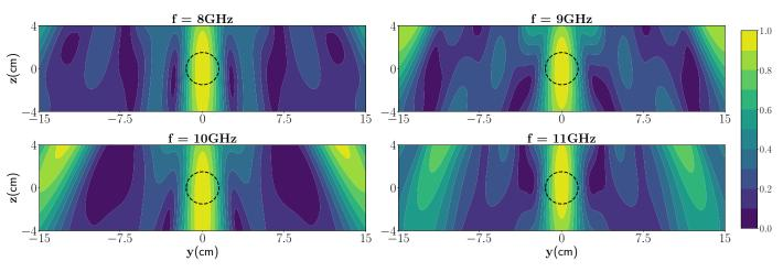
Figure 9. Reconstruction using SF-TRI-DORT at four frequencies.
