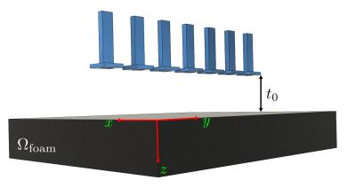
Figure 4. 3-D MWT setup used in this study to generate synthetic measurement data.
