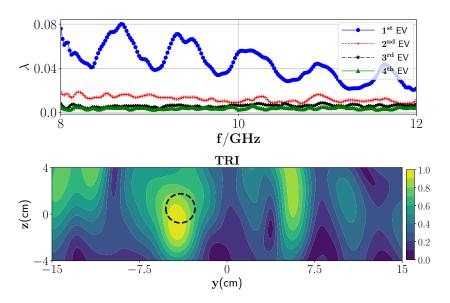
**Figure 14.** (**Top**) Magnitude of the first four eigenvalues versus the frequencies and (**bottom**) TRI-DORT reconstruction image of one wet spot when the second layer is PEC plate.
