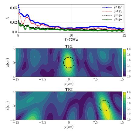
**Figure 6.** (**Top**) Magnitude of the first four eigenvalues versus the frequencies, (**middle**) reconstruction of the first wet spot moisture case with TRI using first dominant eigenvalue, and (**bottom**) reconstruction of the second wet spot moisture case with TRI-DORT using second dominant eigenvalue.
