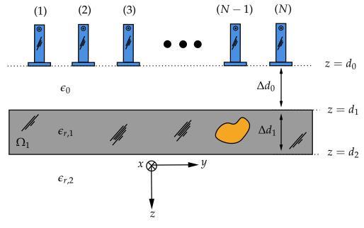
**Figure 2.** Multilayer media with the wet spot(s) in the second layer illuminated by the open waveguide antennas.
