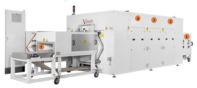
**Figure 1.** A side view of the HEPHAISTOS microwave oven system. Main modules of the oven are represented by number tags 1, 2, 3, 4, 5. Tag 1 and Tag 5 represent the entrance of the wet foam and exit doors for the dry foam on the conveyor belt, respectively. Tags 2, 3, 4 indicate the three modular heating systems which are built into the hexagonal cavity with high power microwave heating sources and control system block.
