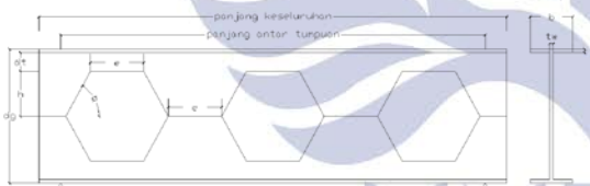
Gambar 3.1. Dimensi Baja Kastela ( castellated beam )
