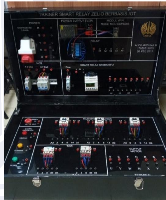
Gambar 3. Desain Trainer Smart Relay Zelio Berbasis Internet of Things .
