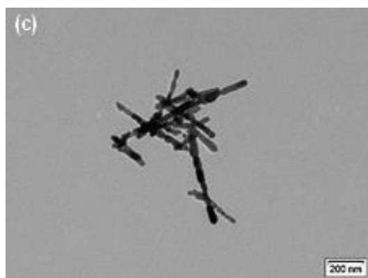
Figure 4 : Bright-field TEM micrographs demonstrating morphology and particle size of the as synthesized (a) \text{NiCo}_2\text{O}_4 , (b) \text{MnCo}_2\text{O}_4 , (c) \text{ZnCo}_2\text{O}_4 .
