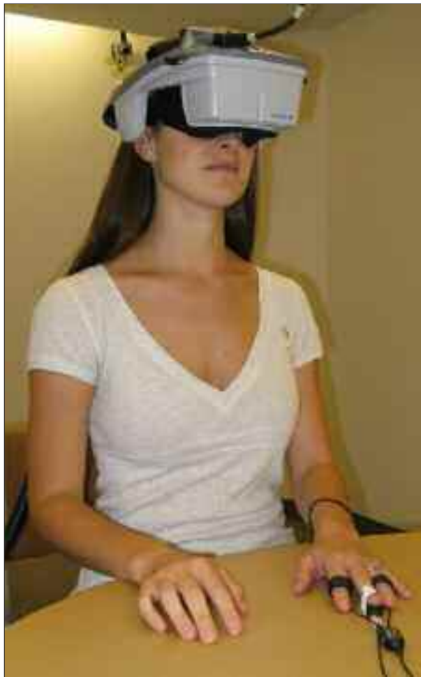
Figure 1. The experimental setup. The participant wears a head-mounted display (HMD) to view the stimulus while the sensors on her hand collect physiological data.
