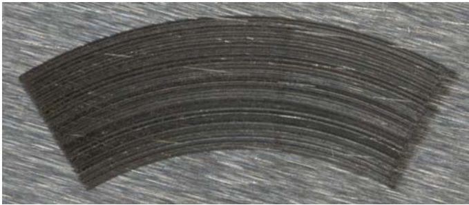
Figure 3.23: Worn cast iron disk used in uncoated test
