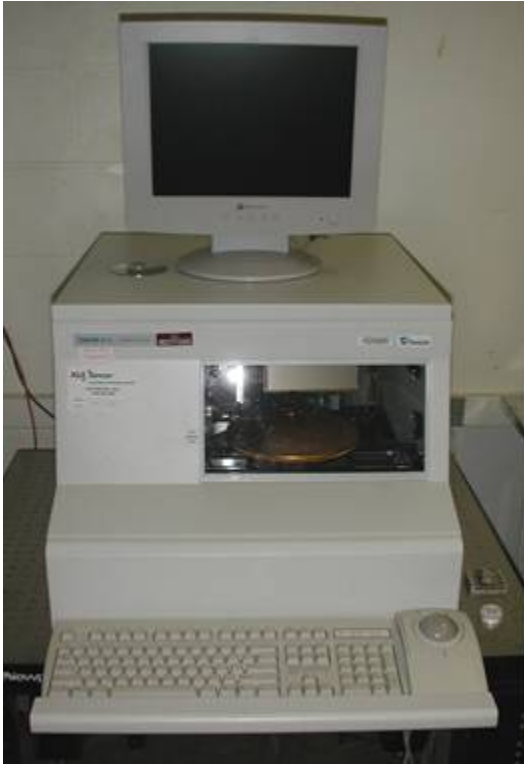
Figure B.1: Tencor P-15 Profiler in Microtribodynamics Laboratory
