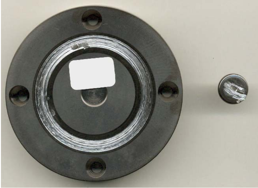
Figure 3.17: Worn CrN + WC/C + DLC coated disk and shoe
