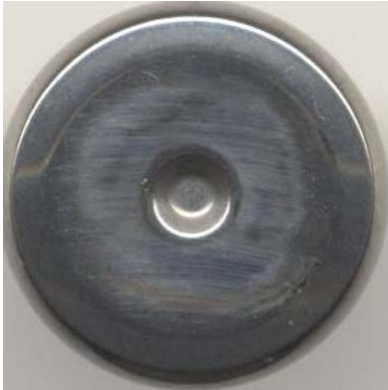
Figure 3.8: WC/C(A) transfer film formed on 52100 steel shoe
