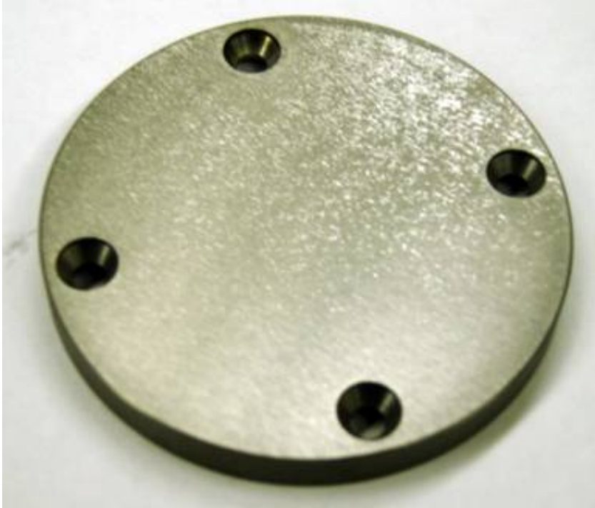
Figure 2.25: Cast iron disk with poor WC/C(A) coating adhesion
