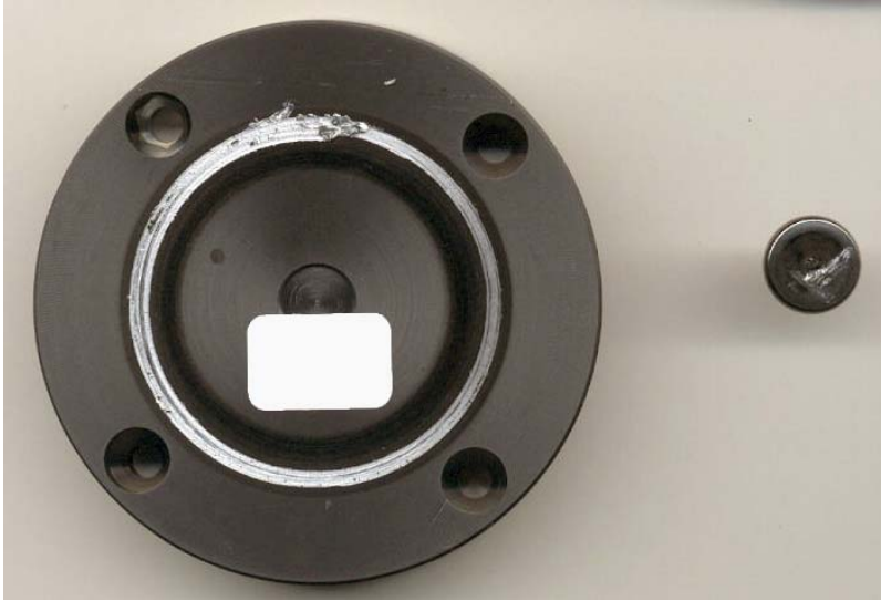
Figure 3.19: Worn WC/C(A) coated disk and shoe
