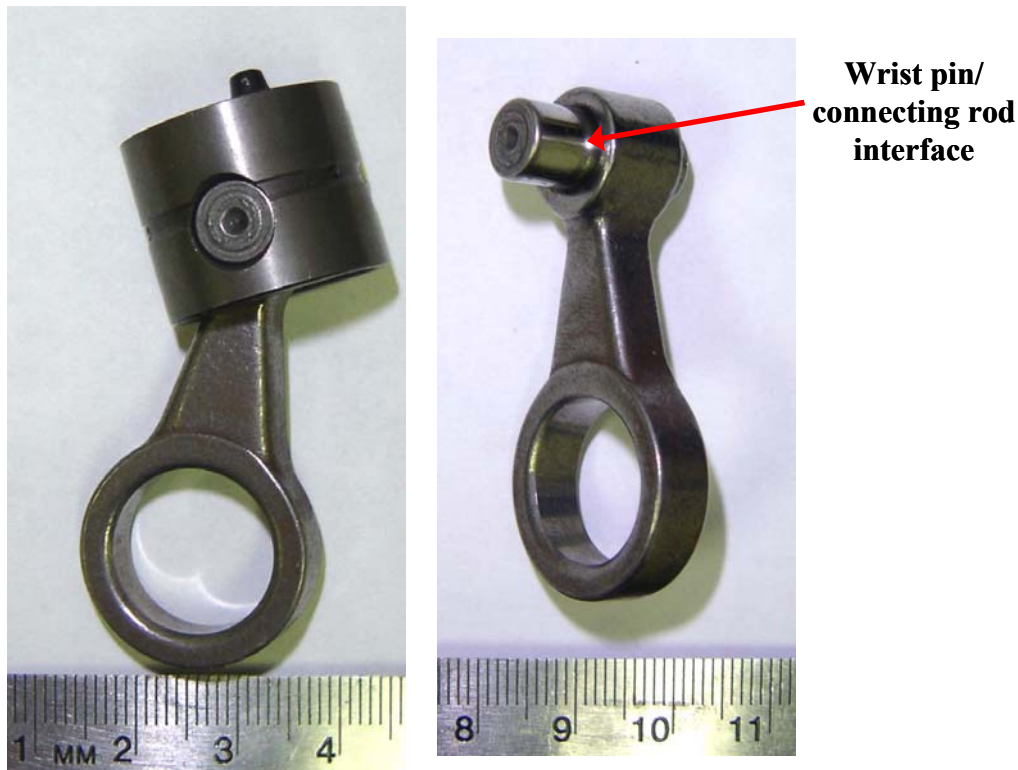
Figure 2.8: Piston assembly for a piston-type compressor indicating the wrist pin-connecting rod interface of interest.
