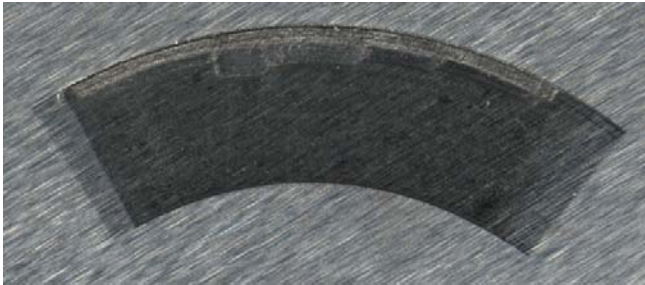
Figure 3.26: Image of worn cast iron disk showing plastic deformation in step-loading test
