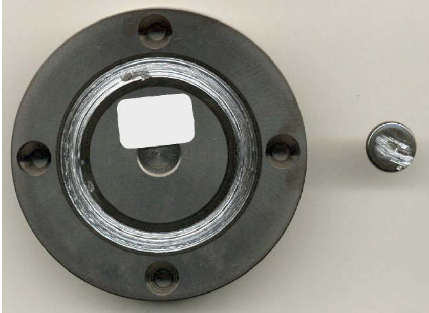
Figure 3.11: Worn CrN + WC/C(B) coated disk and shoe
