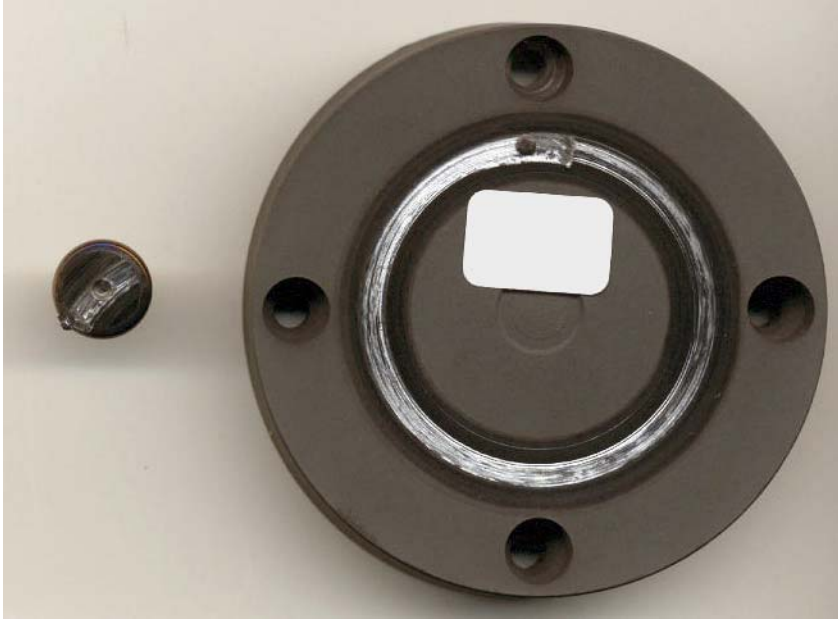
Figure 3.13: Worn CrN + WC/C(A) coated disk and shoe
