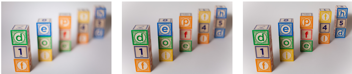
(a) Abertura = f/1,4 , DOF = 0,8cm (b) Abertura = f/4,0 , DOF = 2,2cm (c) Abertura = f/22 , DOF = 12,4cm
