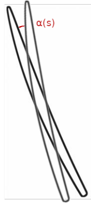
Figure 4.3: Alteration of the blade angle \alpha in function of the sigma-point s .
