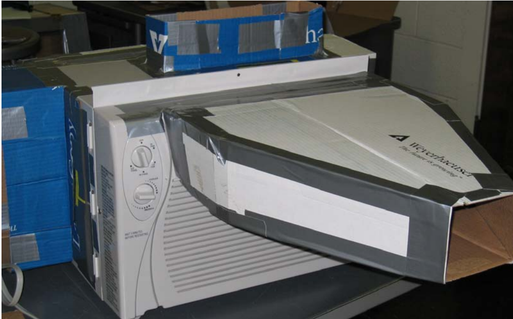
Figure 2.4 Unit while energy balance was performed.
