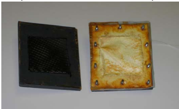
Figure D.8.1 PVC cell with Tyvek membrane stained by Iron chloride.
