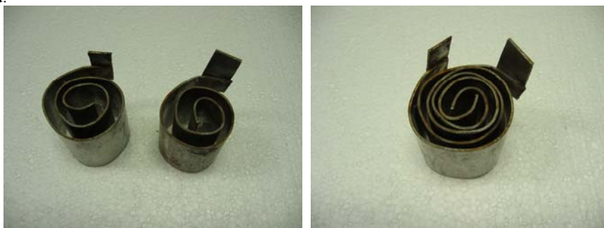
Figure 7.4.1 Chlorine producing cell with stainless steel electrodes. Left: Electrodes separate, Right: electrodes interleaved.
