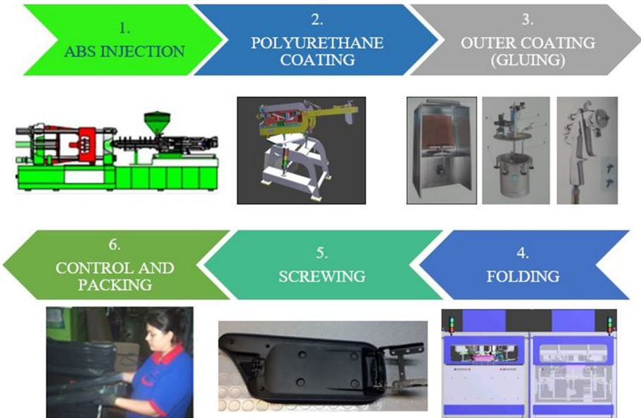
Fig. 2 The production flow of the left armrest
